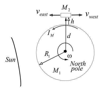
Figure 22: Influence of gravitation on clocks frequency.
