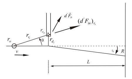
Figure 18: Force induced on a BSP at a bending edge by a BSP moving with speed v.
