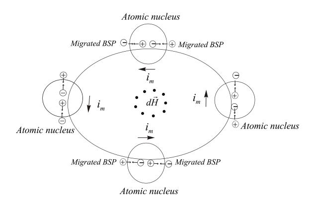
Figure 14: Current flow along a closed chain of reintegrating BSPs
