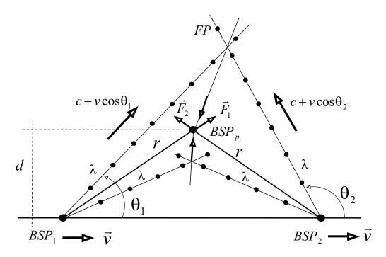
Figure 20: Dragging due to Doppler effect.
