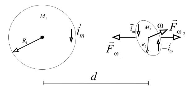
Figure 17: Gyroscopic precession.
