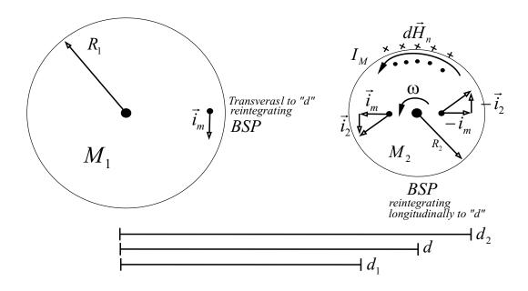
Figure 15: Induced current  $I_M$  and field  $dH_n$  on a rotating neutral body.
